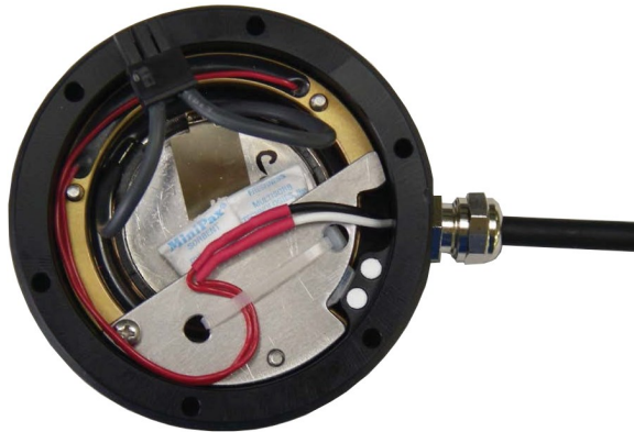
FIGURE D-2. Complete transducer assembly with power connection
